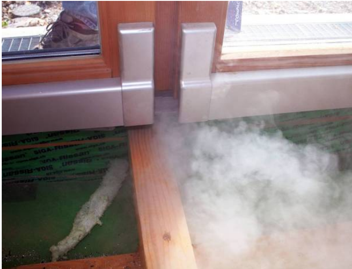
Smoke testing at lift-sliding doors
